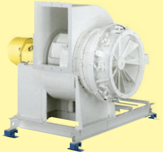
Size 18 Arrangement 1 Class 4 Fan with external inlet damper, unitary base with R-I-S isolation, shaft and bearing guard, belt guard, motor, v-belt drive, and white epoxy coating.
